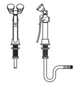
W-0934-00 Deck Mounted Dual Purpose Eye Wash/Drench Hose with two Gentle Spray outlet heads angled at 45° and squeeze valve with locking clip. Flange, shank and locknut for attaching to table top are included. 3/e" I.P.S. male thread swivel inlet.
